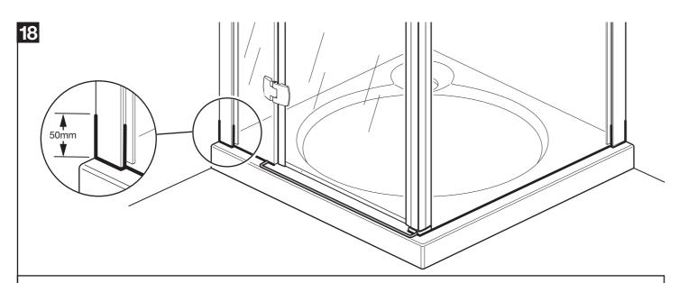
On the OUTSIDE of the enclosure, apply sealant to the bottom of the enclosure and 50mm up the wall channels and vertical joints as shown.
